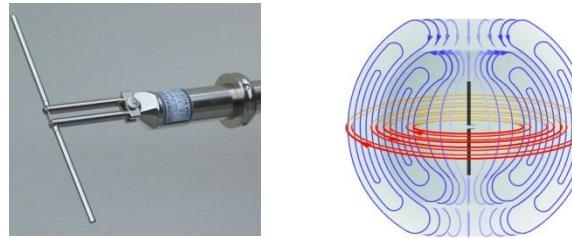
*Dipole Antenna with EM Field of 1.64 mW*
